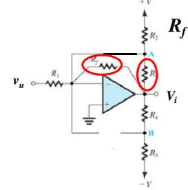
$$R_f' = R_f \parallel R_3 < R_f$$
