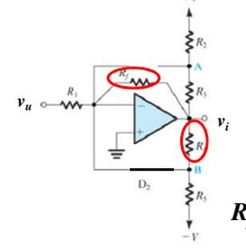
$$R_f'' = R_f \parallel R_4 < R_f$$
